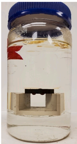
Fig. 3. Contact angle setup used in the research.
