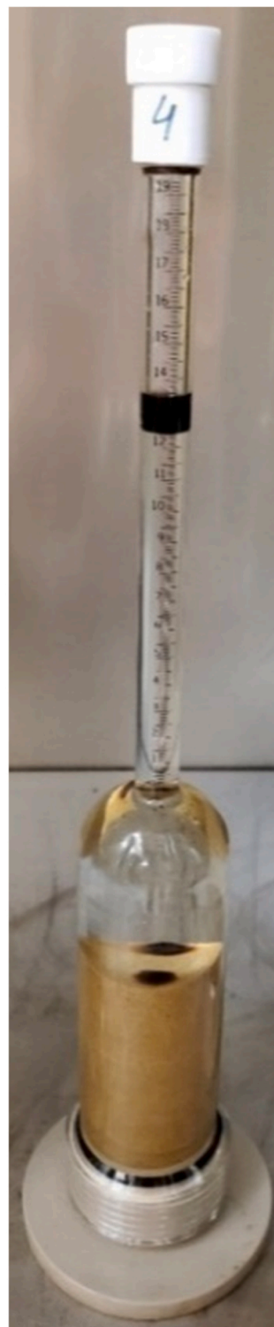
Fig. 4. Amott cell used in the research. An oil aged core was placed in the Amott cell and then the solution to be tested was poured slowly into the Amott cell. All components were at reservoir temperature (347 K) while setting up the experiment to avoid fluid expansion. The produced oil was accumulated at the top and its volume was measured from the grating available on the Amott cell.
