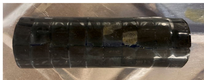
(a) Core pieces #1-#10 were put together for Case 1 (with 0.56-wt% 3pIB)
