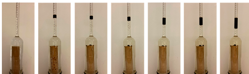
Figure 7. Spontaneous imbibition experiment with 1.07 wt % 3pIB at 338 K.
