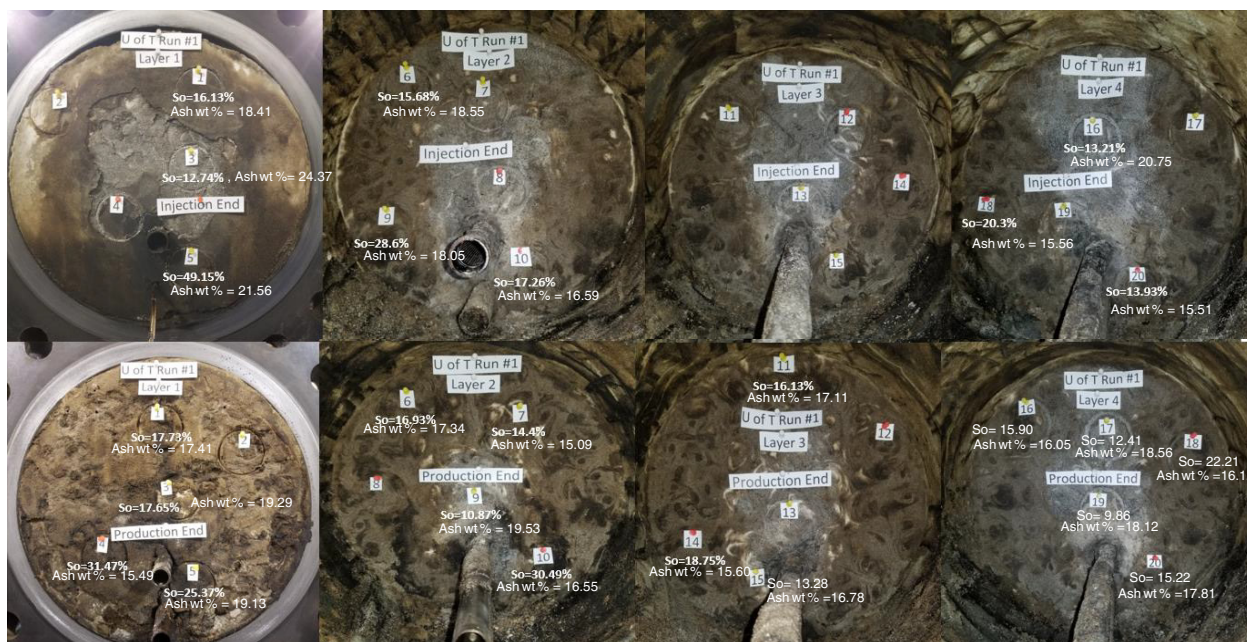
Fig. 10—Photographs of the sandpack after the SAGD experiment. Four pictures at the top are on the injection side, and the four pictures at the bottom are on the production side.
