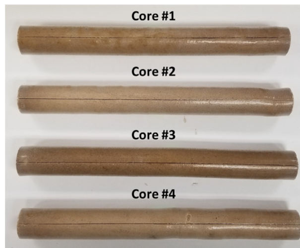
Fig. 2. Artificially fractured Texas cream limestones cores. The diameter is 0.0254 m and the length is 0.229 m. Cores #1 ( S_{wi} = 0 ) and #2 ( S_{wi} = 0.311 ) were used for coreflooding experiments with 3pRB, and cores #3 ( S_{wi} = 0 ) and #4 ( S_{wi} = 0.28 ) with 3p. Table 3 shows the properties of the fractured cores.
