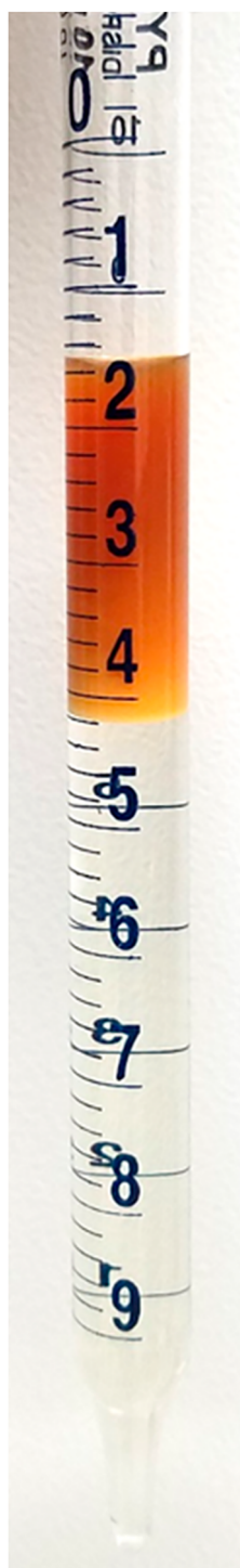
Figure 3. Phase behavior test of the mixture of oil/2-EH-4PO-1SEO/RB at 347 K. The surfactant concentration in RB is 1.0 wt %. The water/oil ratio was 7:3 (i.e., 70 vol % aqueous phase and 30 vol % oil).
