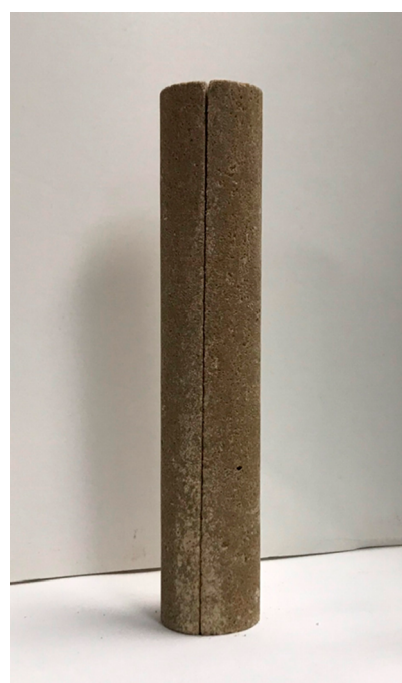
Figure 5. Artificially fractured Indiana limestone core. The diameter is 0.0254 m, and the length is 0.127 m. Table 4 summarizes the properties of fractured cores.
