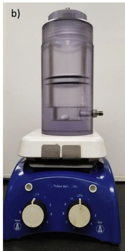
Fig. 1. The new fluid cell made of unfilled polycarbonate placed on a stirring plate.
